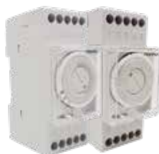
110 0031 - Daily without charge reserve - 2 DIN 110 0032 - Daily with charge reserve - 2 DIN 110 0034 - Weekly with charge reserve - 2 DIN Time switch with tappets with ON/OFF min. 15 minutes
